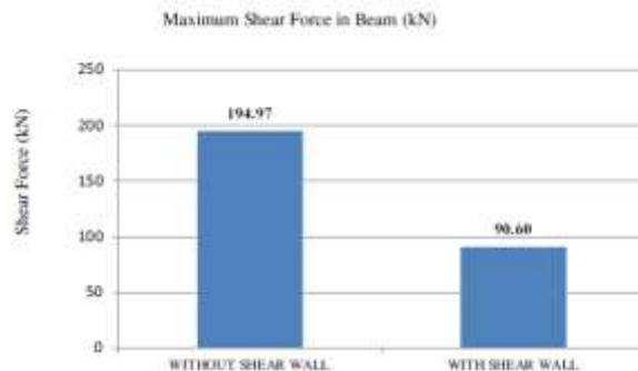
Fig 8 Comparison of maximum shear force
