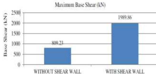
Fig 3 comparison of Maximum base shear
