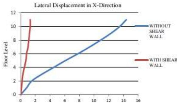
Fig 4 Comparison of lateral displacement in x-direction
