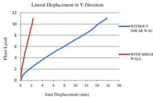
Fig 5 Comparison of lateral displacement in y-direction
