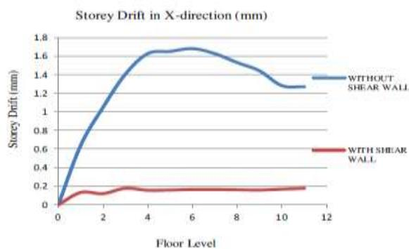
Fig 6 Comparison of storey drift in x-direction
