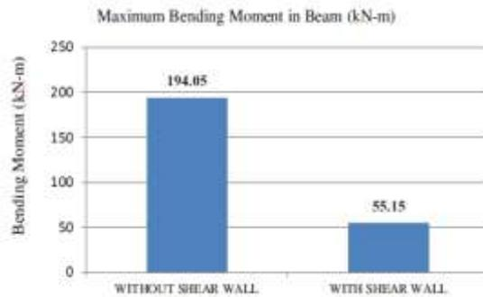
Fig 7 Comparison of maximum bending moment
